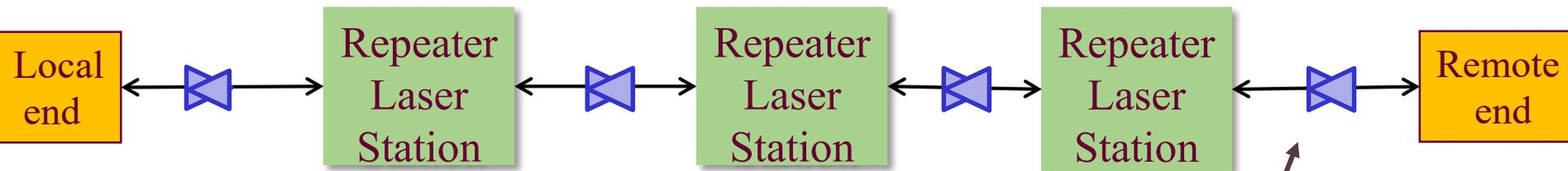
Repeater station N, including a regeneration laser: send back signal to station N-1, amplify and filter, correct the noise of next link N
