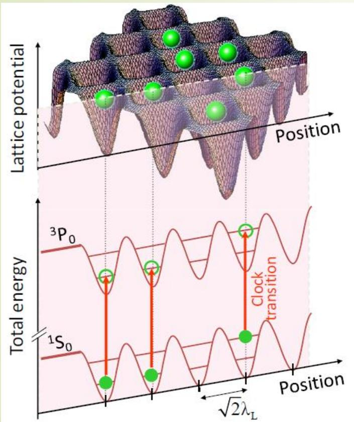
Optical lattice potential confines millions of neutral atoms in separate micro-traps
