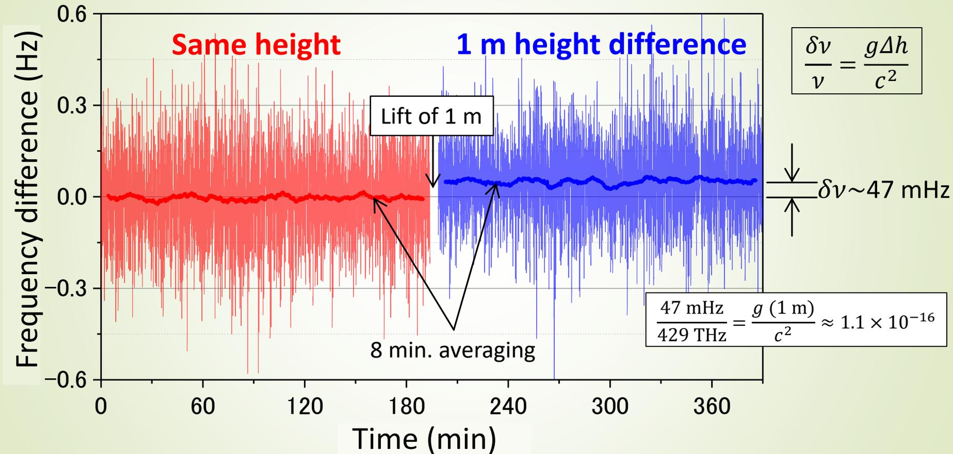
Time dilation for 1 m height difference due to general relativity is resolved by comparing optical lattice clocks with a few minutes of averaging time
